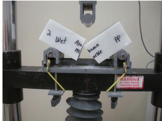
Photo No. 6 ASTM C99 – Representative Specimen Failure Mode
