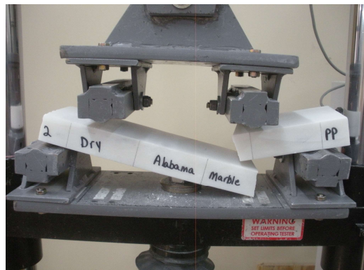
Photo No. 8 ASTM C880 – Representative Specimen Failure Mode
