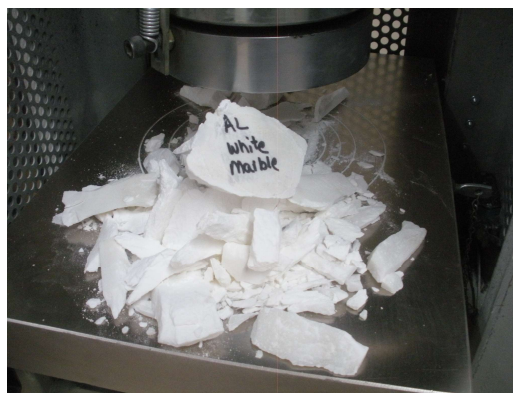
Photo No. 4 ASTM C170 – Representative Specimen Failure Mode
